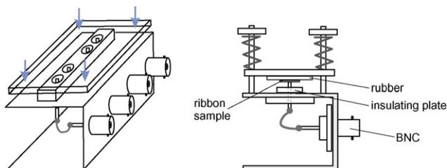
Fig. 1. The sample holder used for magnetoimpedance measurements.
