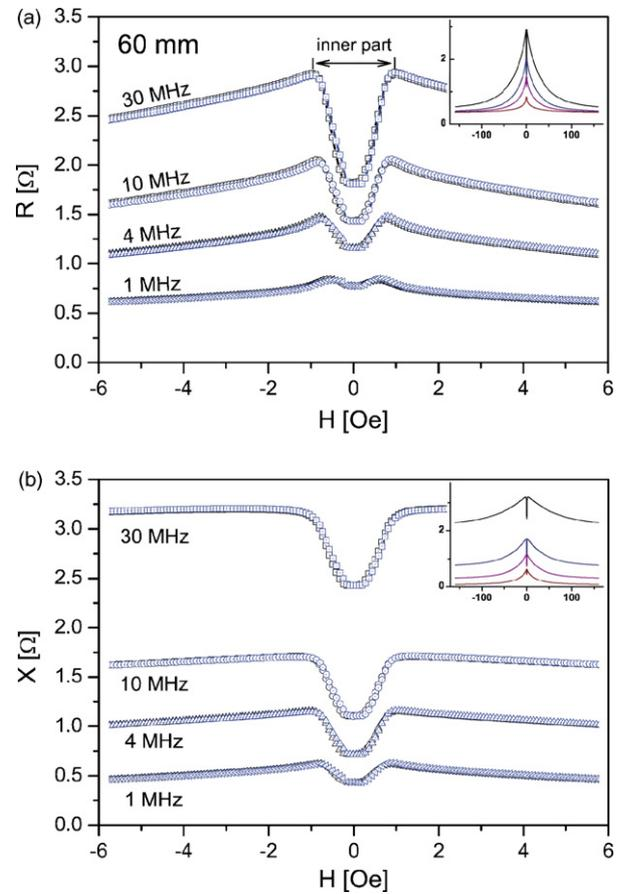
Fig. 2. Field dependence of the real (a) and imaginary (b) components of the impedance of L1-sample.
