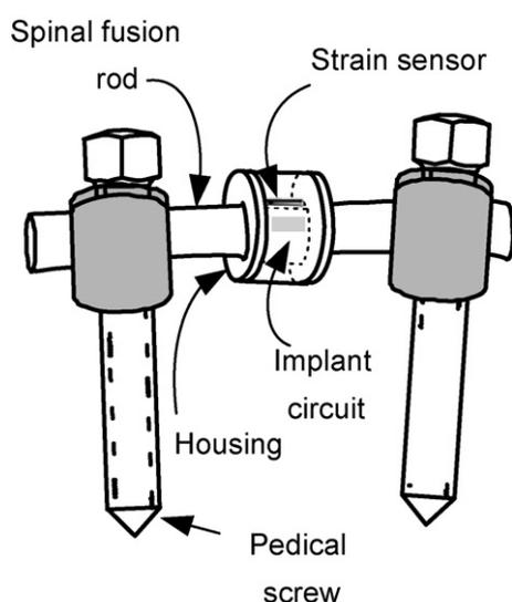
Fig. 2. The SFMI implant attached to a spinal fusion rod.
