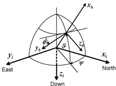
Fig. 2. Orientation of the body frame expressed in the inertial frame.
