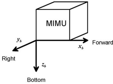
Fig. 1. Body frame fixed to the MIMU's casing.
