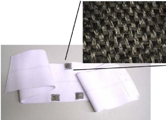
Fig. 2. Belt with Textrodes.
