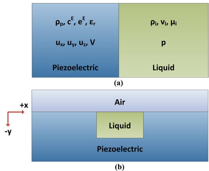
**Fig. 1.** (a) A schematic representation of the important domains in the model. The characteristics of the media and independent variables are indicated. (b) Depiction of the 2D version of the real problem to be solved with the cavity. The air–liquid and air–piezoelectric boundaries can be simplified and neglected due to negligible acoustic transmission coefficient between these two pairs of media, hence eliminating the air domain completely.
