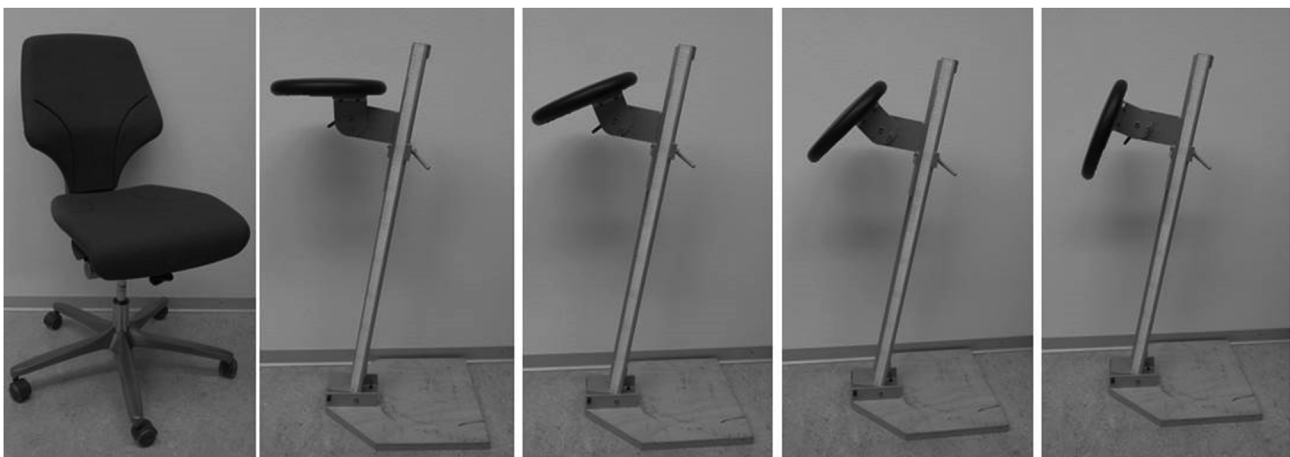
Fig. 1. The office chair and the prototype of the sit-stand-support with the angles 0^\circ to the horizontal axis, 25^\circ , 50^\circ and 65^\circ . The height of the devices that was chosen by the subjects was 21.0\% \pm 1.4\% body height, 40.0\% \pm 1.4\% body height, 43.0\% \pm 1.6\% body height, 46.2\% \pm 1.4\% body height and 50.1\% \pm 1.5\% body height from the left to the right.
