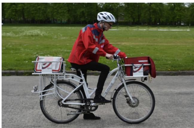
Fig. 1. The current electrically assisted bicycle of bpost, which was introduced approximately six years ago. Front carrier can hold 1 bag, rear carrier can hold 2 full bags and 6 empty bags of mail.
