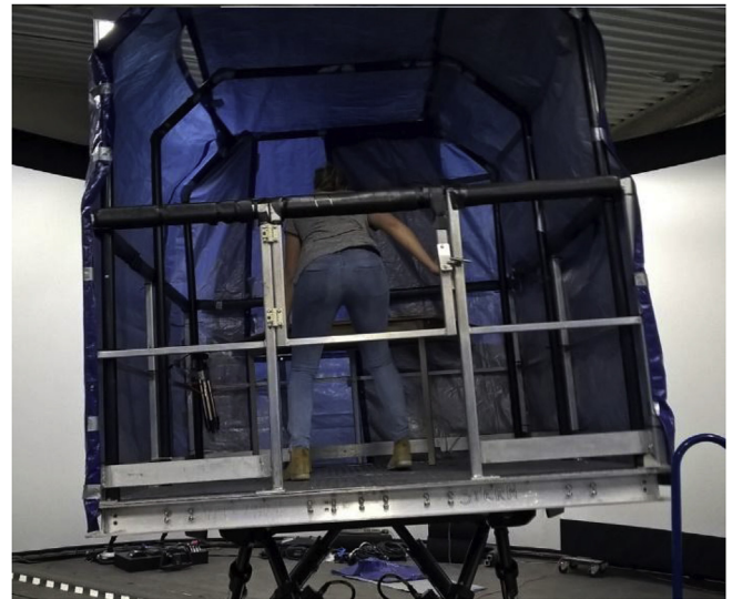
Fig. 1. Picture showing the motion simulator and setup used for the study. A table can be seen in front of the participant while he or she faced forward, unable to see outside of the simulator as a result of the cover.
