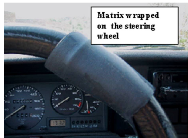
Fig. 2. Capacitive sensor matrix in the operator's hand position.
