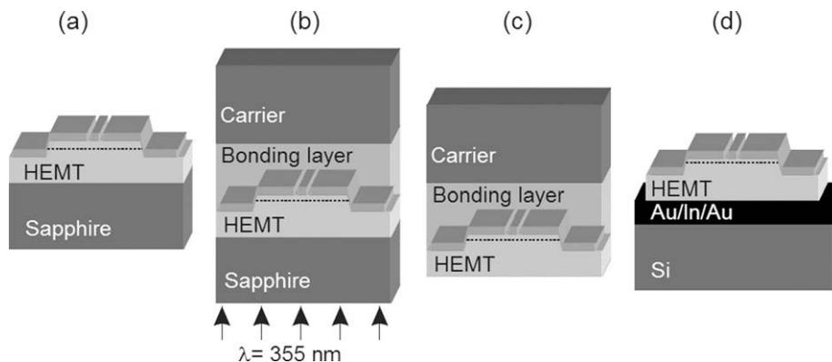
**Fig. 1.** Schematic of AlGaIn/GaN HEMT LLO transfer process: (a) as-grown HEMT on sapphire substrate, (b) bonding to carrier and application of laser pulses to sapphire substrate backside, (c) removal of sapphire substrate, and (d) bonding to Si substrate and carrier removal.
