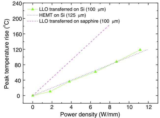
**Fig. 2.** Peak temperature rise in an LLO transferred AlGaIn/GaN HEMT onto Si, compared to device directly grown on Si (from Ref. [2]). Results on an LLO transferred AlGaIn/GaN HEMT onto a new sapphire substrate is also included. Gate width for all devices was 100 μm, apart from the device on Si which was 125 μm.
