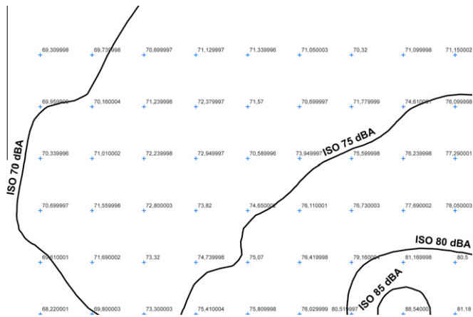
Fig. 1. Contour lines obtained by interpolation of sampling grid.
