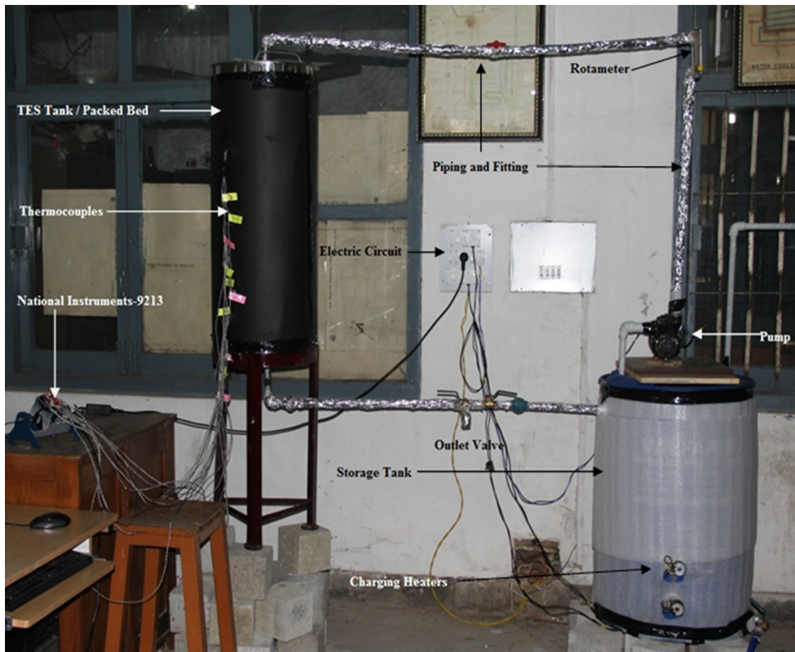
Fig. 1. Complete experimental set-up.
