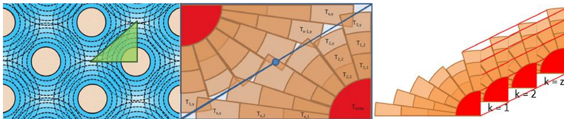
Fig. 1. Grid layout of shell-and-tube matlab model. (a) Overall heat exchanger geometry, (b) Boundary conditions for quarter tube calculation domain, (c) longitudinal direction.
