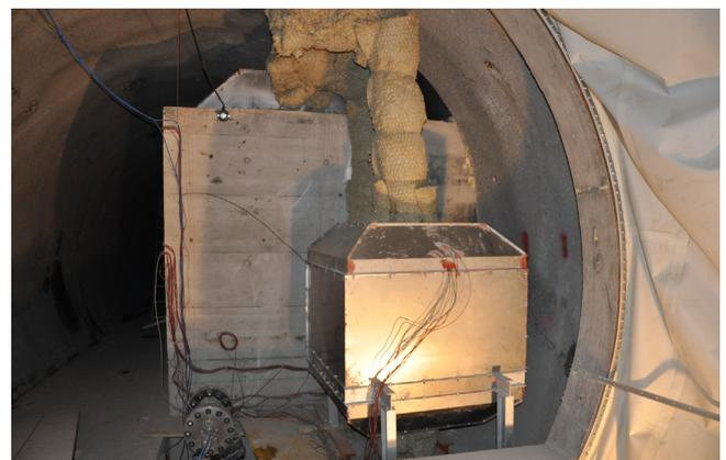
**Fig. 1.** Picture of combined sensible/latent TES, with latent storage in foreground and sensible storage in background. The insulated pipes between the heater and the latent storage and between the latent and sensible storages can be seen.
