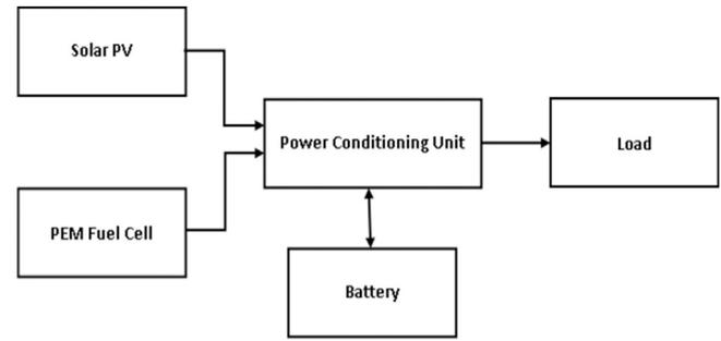
Fig. 1. Block diagram of solar PV- PEM fuel cell based integrated energy system.
