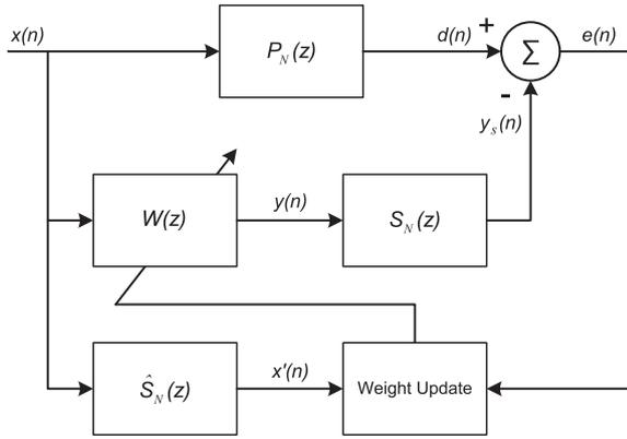
Fig. 1. Block diagram of an FxLMS algorithm based ANC system.
