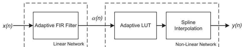
Fig. 2. Linear non-linear network.
