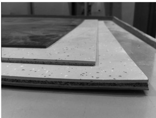
Fig. 1. The 3 commercial resilient surface layers under test.
