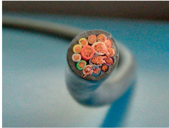
Fig. 1. Real multicable with 15 single cables.
