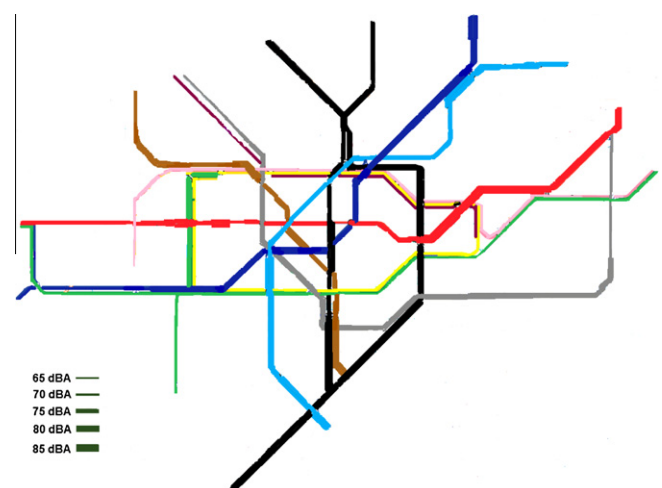
Fig. 1. Noise levels (dBA) measured across a metro transport network on train carriages showing levels from 65 to 85 dBA.
