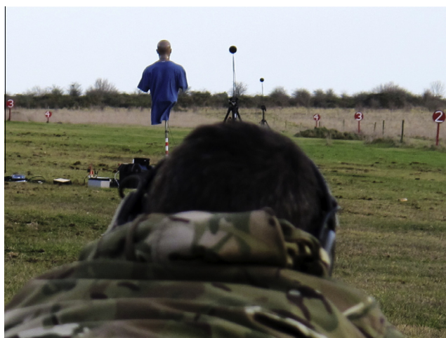
Fig. 3. View, from behind the firer, of the Kemar manikin with the quarter-inch microphone to the right. (The more distant microphone was not in use.)
