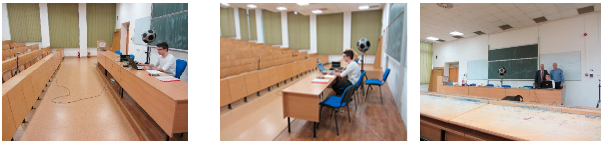
Fig. 2. Images from the acoustic measurements in the Lecture Hall.
