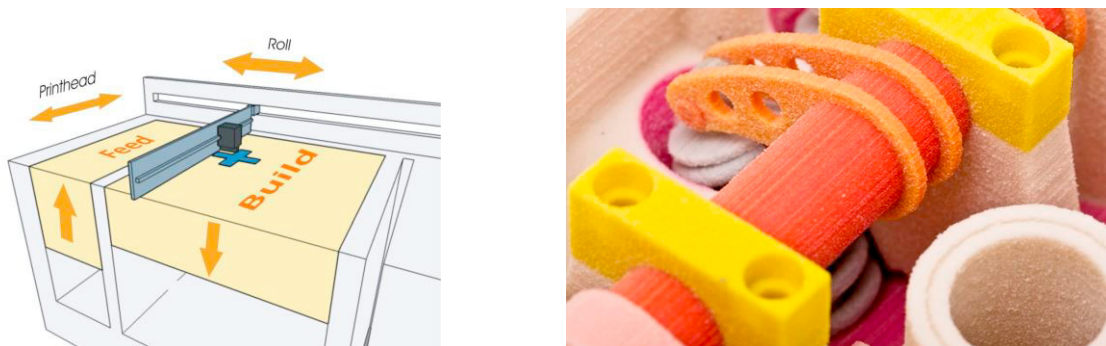
Fig. 1: (a) 3D printing process principle [2], (b) multi-coloured 3D printing example part [3]
