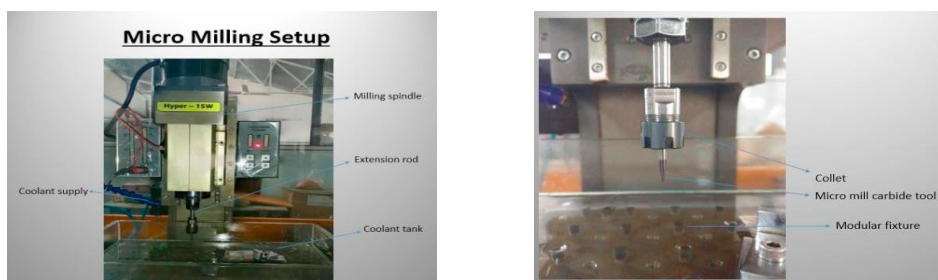
Fig .1. (a) Micro milling setup; (b).Collet and modular fixture arrangement
