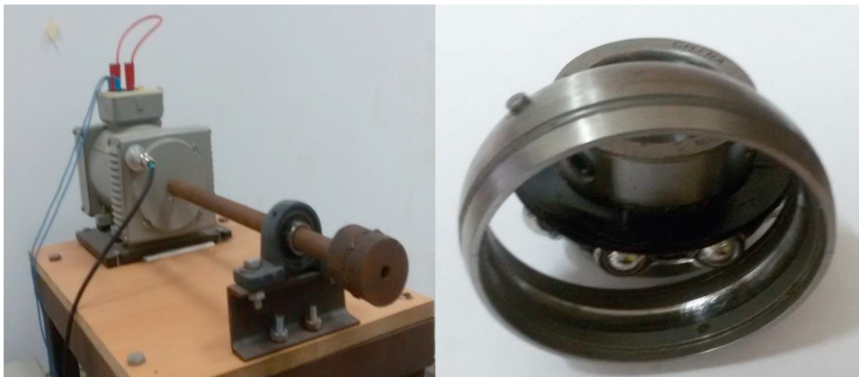
Figure 1 Experimental test rig and rolling element ball bearings
