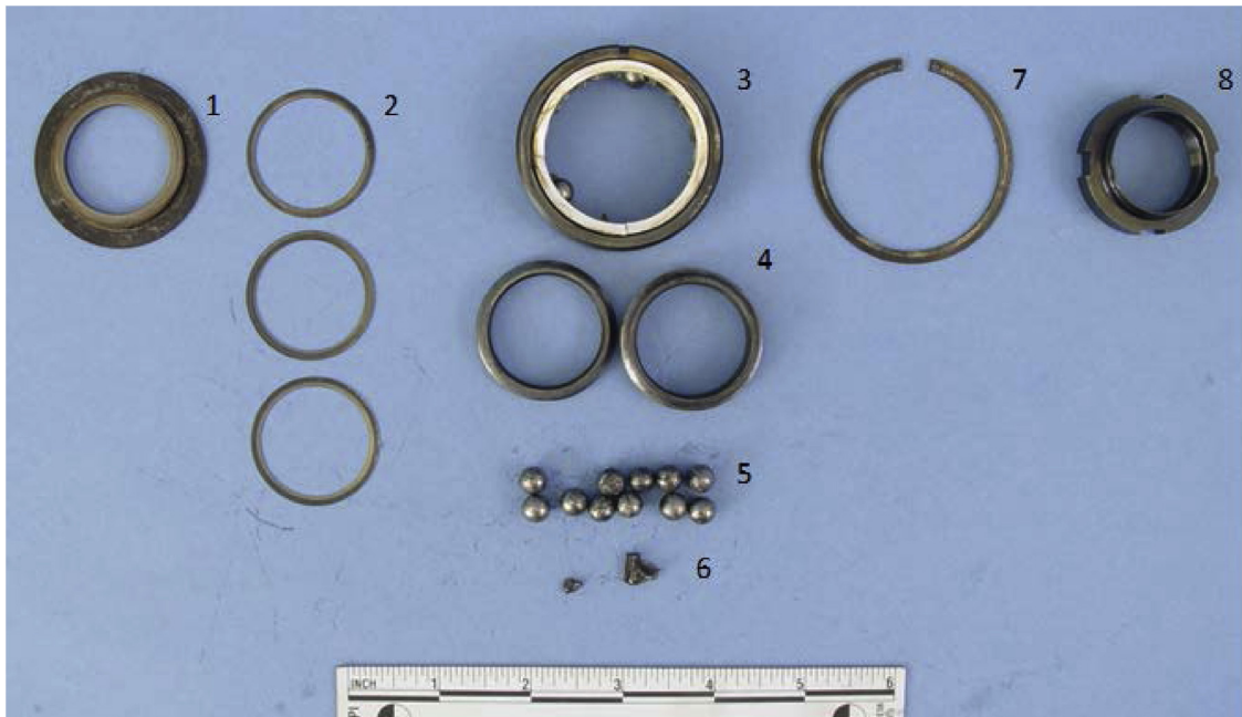
Fig. 1. Picture of the as-received No. 2 bearing pieces, oil slinger, shims, retaining ring, and spanner nut as identified in the following list: (1) oil slinger, (2) shims, (3) No. 2 bearing piece (outer race, retainer pieces, and two balls), (4) No. 2 bearing inner race halves, (5) eleven bearing balls, (6) bearing retainer pieces, (7) retaining ring, (8) spanner nut.
