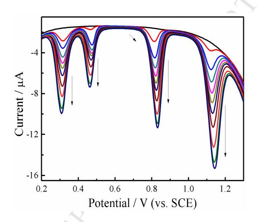
Shown up were DPVs of poly(glycine)/graphene oxide modified electrode for the simultaneous determinations of dopamine, uric acid, guanine and adenine.
