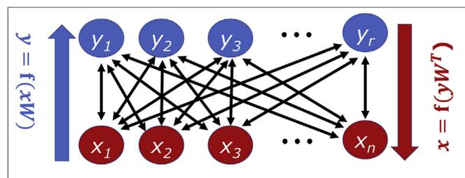
Fig. 1. Schematic of an RBM bipartite bidirectional network. The  $n$  input units are the red circles (i.e., spectra) and the  $r$  hidden units (i.e., features) are the blue circles. The connection strengths are stored in the weight matrix  $\mathbf{W}$ , which is used to propagate signals in the forward (up) and backward (down) directions. (For interpretation of the references to colour in this figure legend, the reader is referred to the Web version of this article.)
