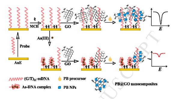
Schematic illustration of the sensor fabrication process and the generation of prussian blue nanoparticles on graphene oxide sheets used as electrochemical signal label for As(III) detection.
