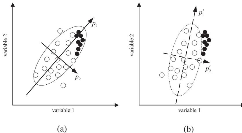
Fig. 1. PCA (a) and ASPCA (b) on data with variables 1 and 2 in two operating conditions. The variables are independent in the normal operating condition (○), but correlated in the current operating condition (●).
