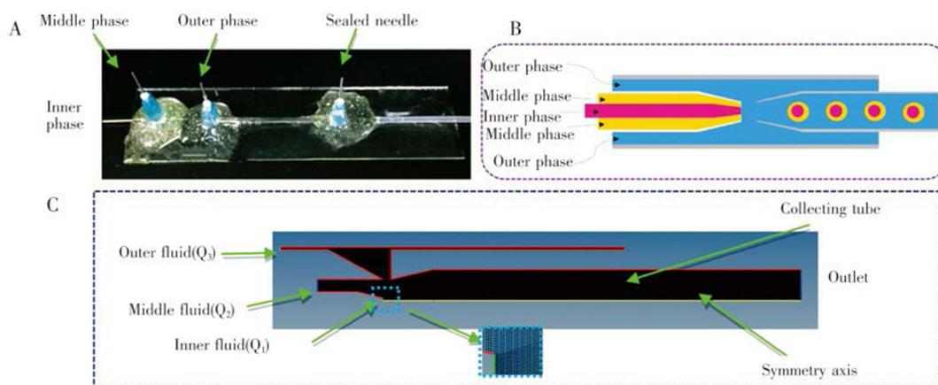
Fig.1 Microfluidic chip structure diagram for synthesis of double emulsion droplets: (A) glass capillary microfluidic device; (B) schematic illustration of double emulsion generation process; (C) schematic of simulated mesh
