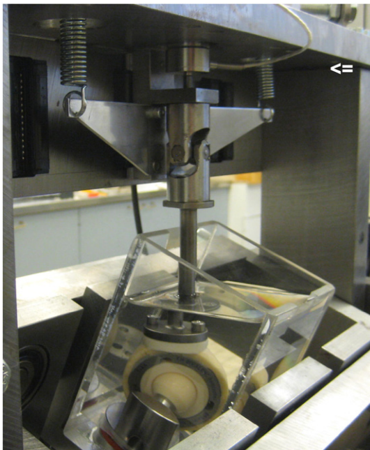
Fig. 2. Separation mechanism, operated by vertical springs and counter-pressure on piston rod side of pneumatic loading cylinder of the HUT-4 hip joint simulator. In this system test with 28\text{ mm} AoA, cup inclination angle was 64^\circ , lift height (vertical separation) was 1.0\text{ mm} , and lubricant was distilled water. Arrow indicates where spacers are placed for adjustment of vertical separation.
