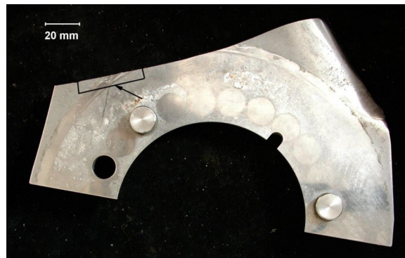
Fig. 1. General view of the broken blade. The arrow indicates the place where sample was taken for testing and indicates the place where the inscription (number "1") was made with engraving tool.
