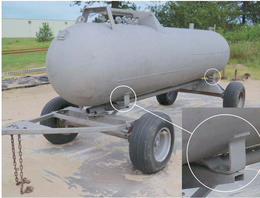
Fig. 1. Anhydrous ammonia nurse tank mounted on running gear. Inset shows that the leg attachment brackets are welded directly to the tank body to connect the tank to the running gear.
