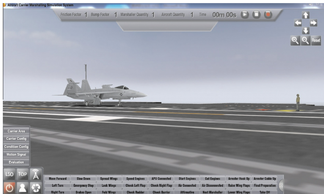
Fig. 1 PC-based aircraft carrier marshalling simulation training system interface.
