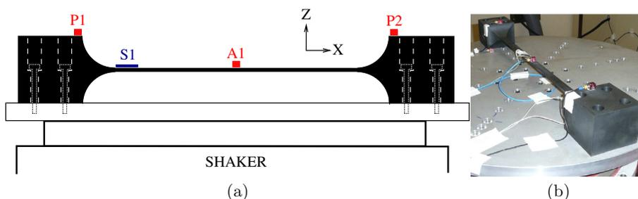
Fig. 1. A schematic (a) and a picture (b) of the experimental setup which includes 3 accelerometers (P1,P2,A1) and a strain gage (S1).
