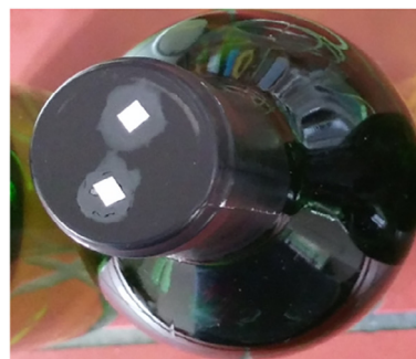
Fig. 1. Sealing of the holes on the top of the capsules by aluminum folia pieces and EVOH polymer (example of Al-pol capsule).
