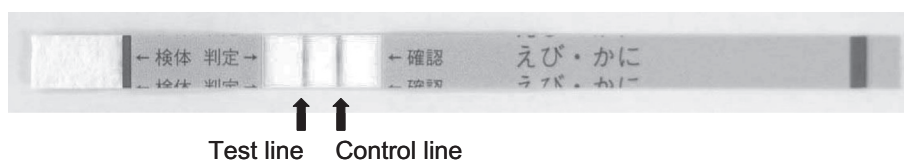
Fig. 1. The lateral flow device. When test and control lines appear, the sample is positive. If test line does not appear, the sample is negative.
