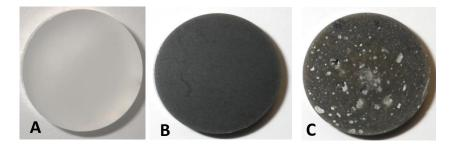
Disks prepared from resin/hardener: A) blank (no sample), B) with BCR-2 powder under vacuum, and C) with BCR-2 powder in air. Bubbles are formed when resin impregnation takes place in air due to the evolution of interstitial air between powder grains.
