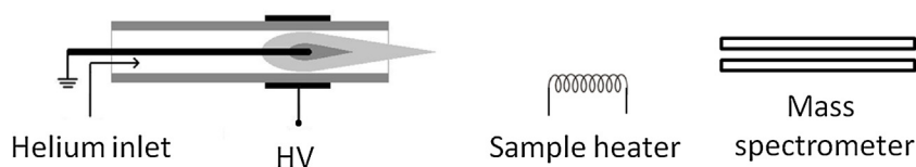
Fig. 1. Schematic diagram of DBDI source with sample heater.
