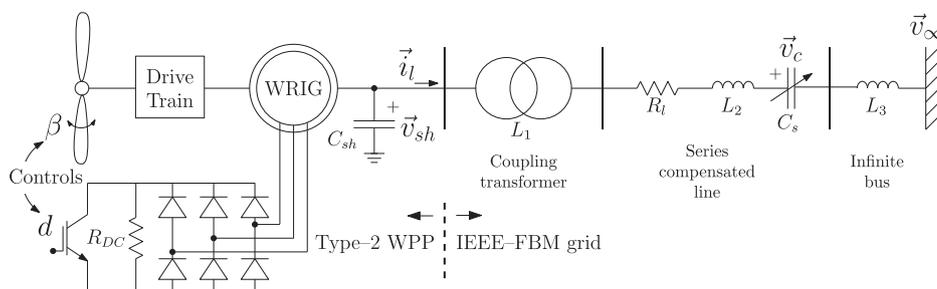
Fig. 1. Schematic of the power system under study. The IEEE-FBM for SSR analysis has been modified replacing the synchronous generator by a Type-2 WPP [23].
