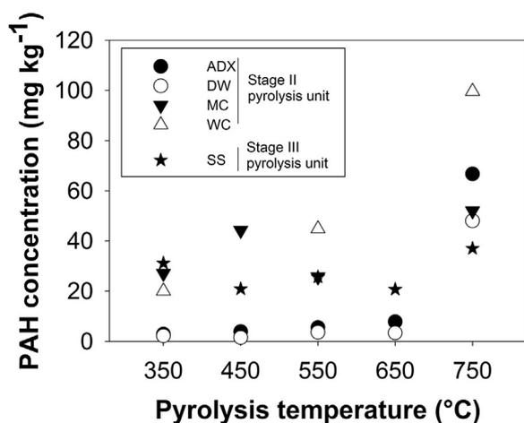
**Fig. 1.** Effect of pyrolysis temperature on 16 US EPA PAH concentration in biochar ( $\text{mg kg}^{-1}$ ). The biochars were produced from 4 different feedstocks in Stage II pyrolysis unit (ADX, *Arundo donax*; DW, demolition wood; MC, miscanthus chips; WC, willow chips) and 1 feedstock in Stage III pyrolysis unit (SS, sewage sludge). For all the feedstocks combined, the PAH concentration in the biochars produced at 750 °C is significantly different to all the other HTTs (one-way ANOVA).
