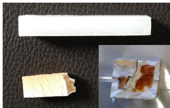
Fig. 1. Picture of the new PE sample (top) and the aged sample (bottom left and right).
