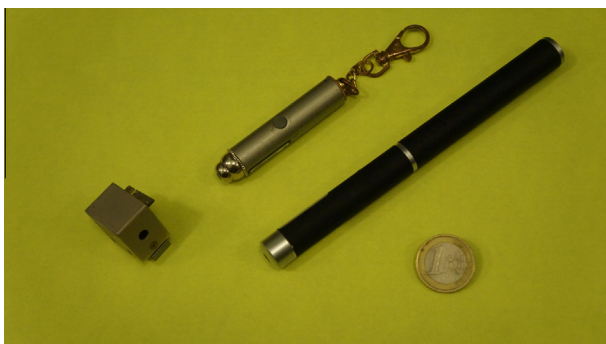
Fig. 1. Photo of the acousto-optic filter together with the “red” (short) and “violet” (long) laser pointers.
