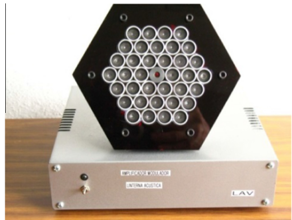
Fig. 1. A photograph of the parametric source with the electronics housing is shown. In this case, the central source was substituted with a laser diode from a laser pointer. The data measurements were obtained with the central source in place.
