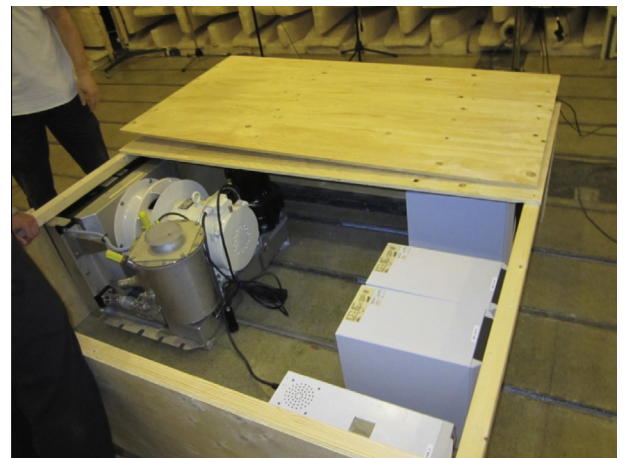
Fig. 1. A centrifugal fan inside the mock-up. The computer cases are used to reduce the size of the outlet.
