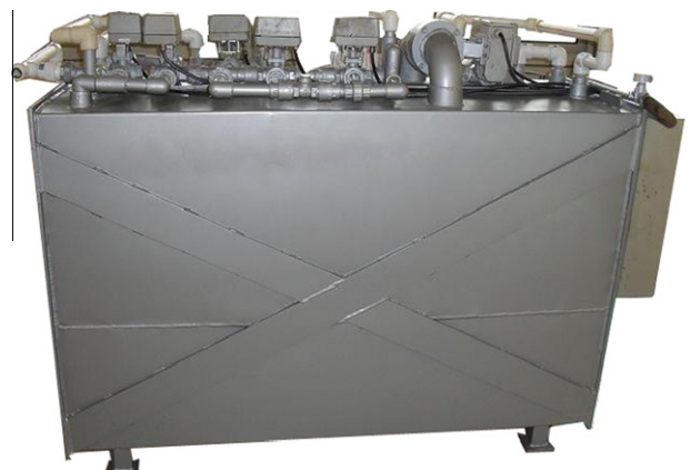
Fig. 2. The picture of adsorption cooling machine (there are two machines, silica gel-water was used for chiller in one machine, and silica gel/LiCl-methanol was used for refrigerant in the other machine).
