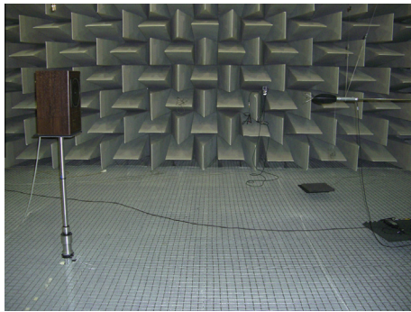
Fig. 2. Frequency response measurement setup.
