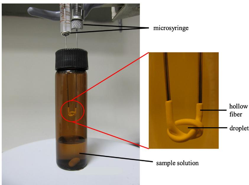
Fig. 1. The extraction equipment of HS-K-HFME.
