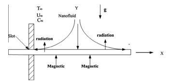
**Fig. 1.** A sketch of the physical model for nanofluid toward an extrusion stretching sheet with magnetic and radiation energy conversion conjugate heat and mass transfer system.
