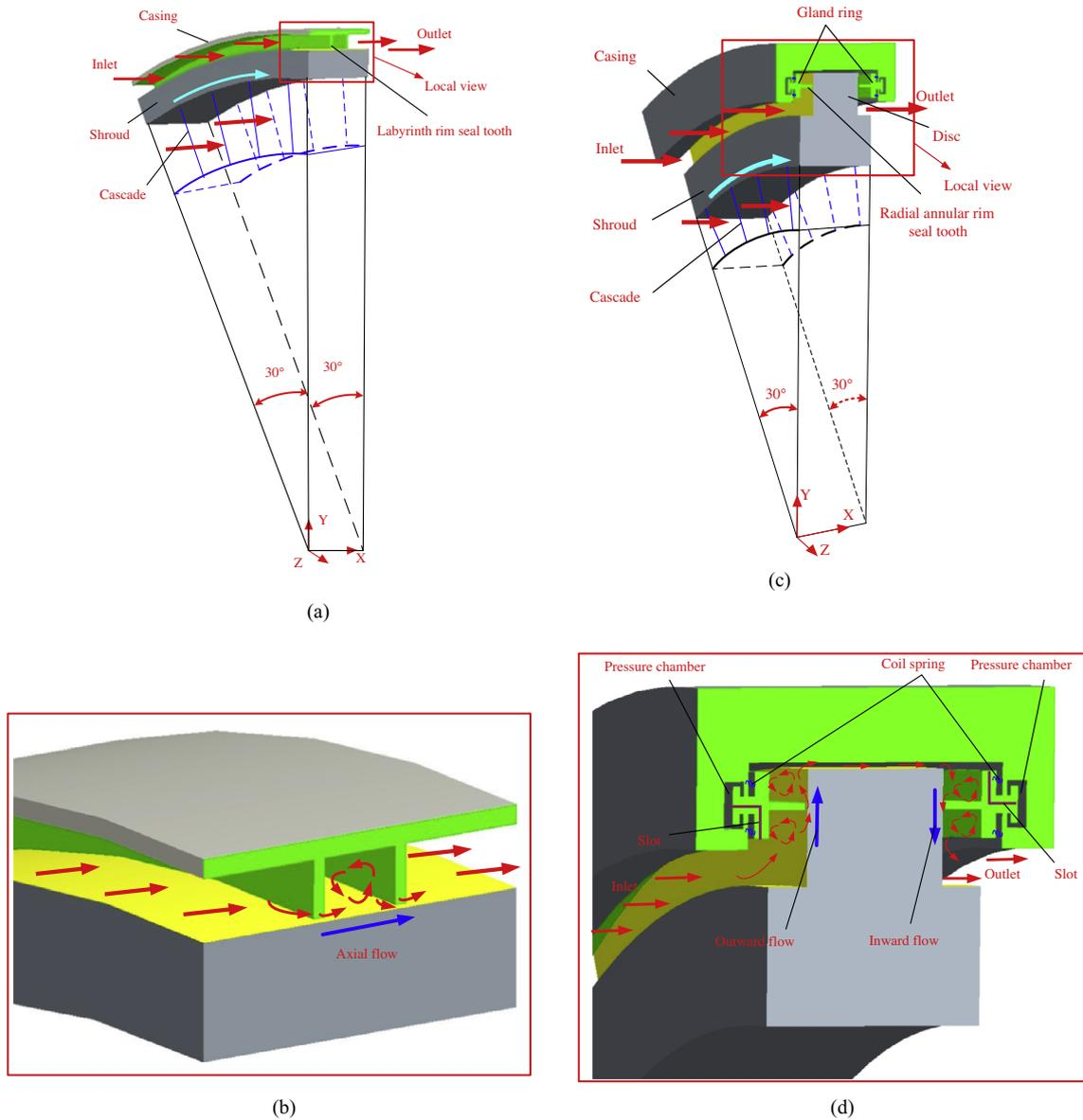
**Fig. 1.** Schematic structure of the LRS and the RARS. (a) Entire structure of the LRS. (b) Local view of the LRS. (c) Entire structure of the RARS. (d) Local view of the RARS.
